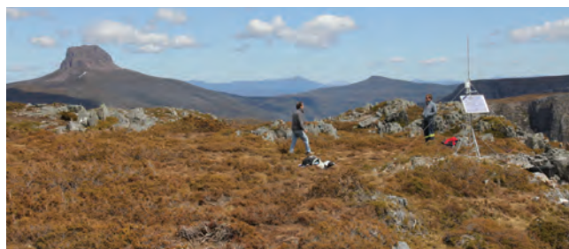
A weather site installed on Cradle Plateau (Barn Bluff behind) to monitor soil and air temperature and moisture parameters to address climate change research gaps in Tasmania. Photo Micah Visoiu
